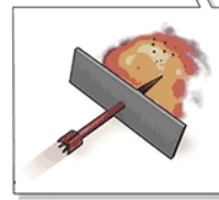
Depleted uranium penetrator with stabilizing fins
